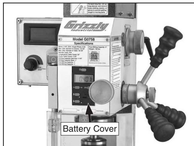
Figure 43. Battery cover for DRO.
