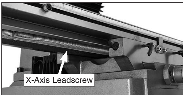
Figure 39. Location of X-axis leadscrew.
