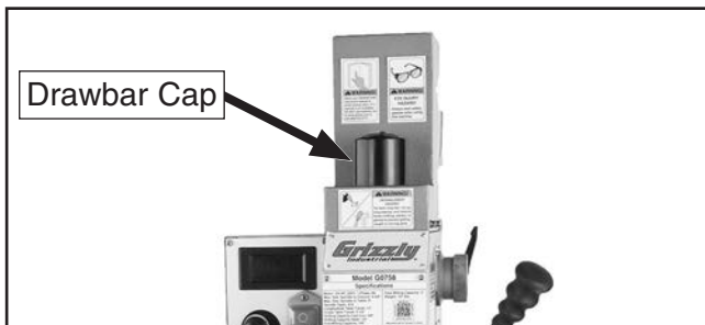
Figure 27. Location of drawbar cap.
