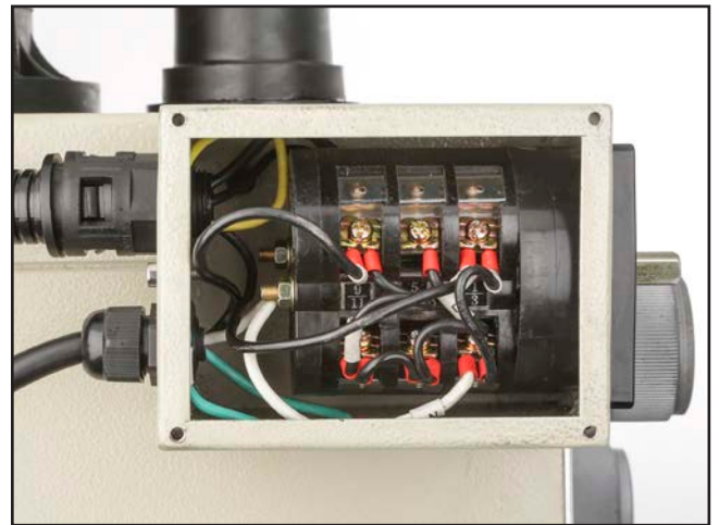
Figure 49. Switch box wiring.
