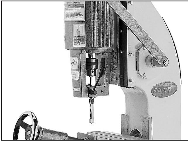
Figure 18. Auger bit and chisel correctly installed.
