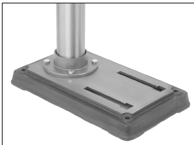
Figure 7. Column secured to base.
