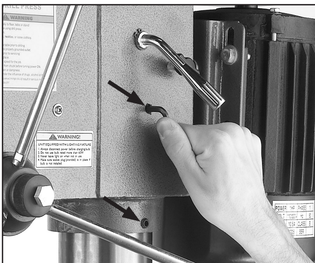
Figure 14. Securing headstock to column.
