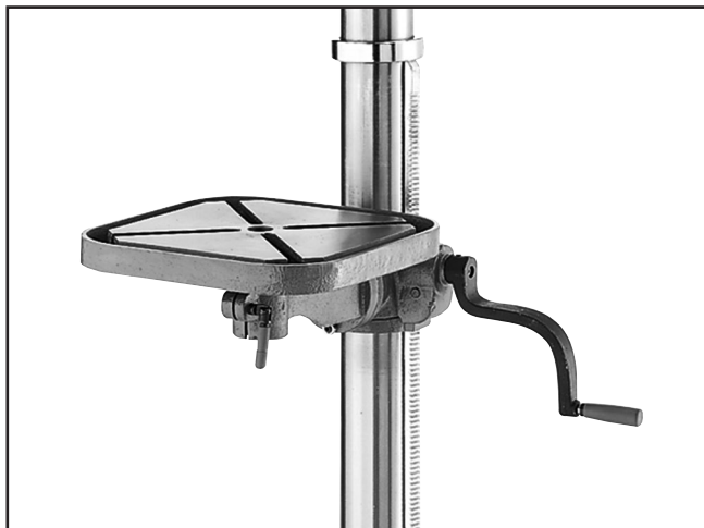
Figure 19. G7947 table installed.
