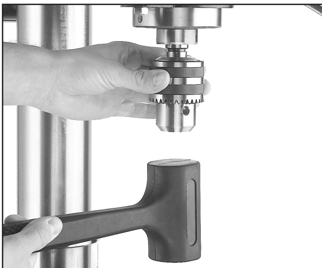
Figure 17. Seating arbor and chuck into spindle.
