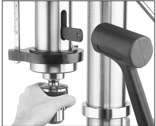
Figure 32. Using drift key to remove arbor.
