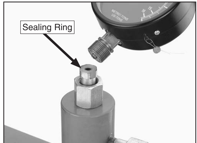
Figure 16. Hydraulic line installation.
