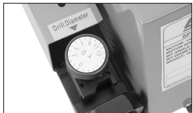
Figure 11. Calibrating dial set for a 7mm drill bit.
