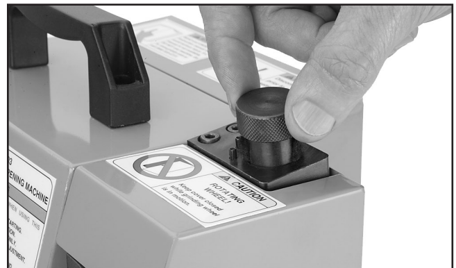
Figure 27. Cleaning rear trimming area.
