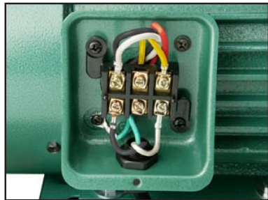
Junction Box @ 110V.
