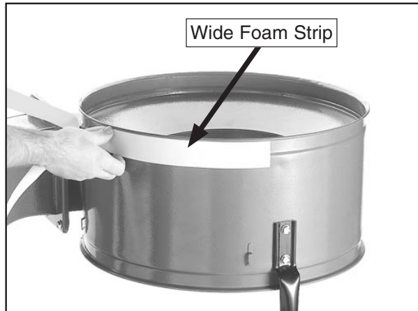
Figure 20. Applying the wide foam strip to the collector.
