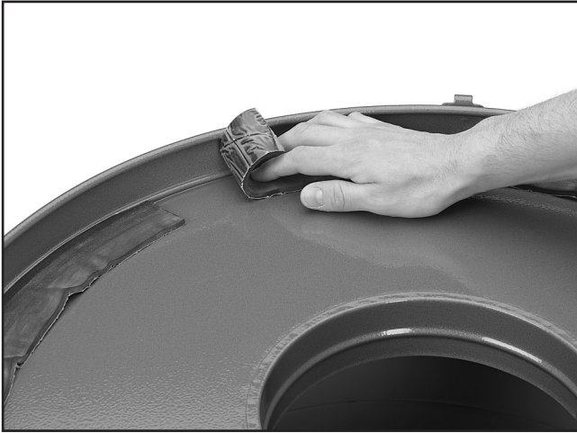
Figure 34. Applying dust collection drum lid gasket.
