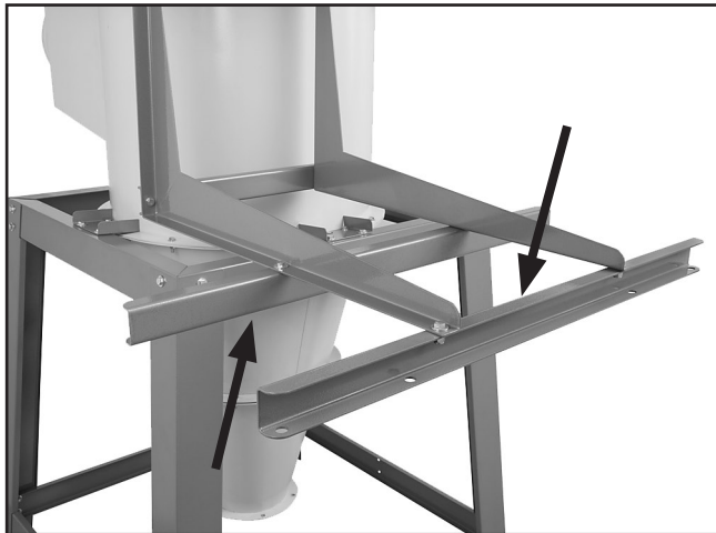
Figure 27. Long brace supports attached.
