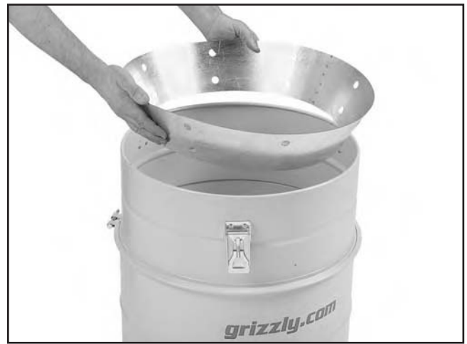
Figure 23. Installing the dust collection bag seat.
