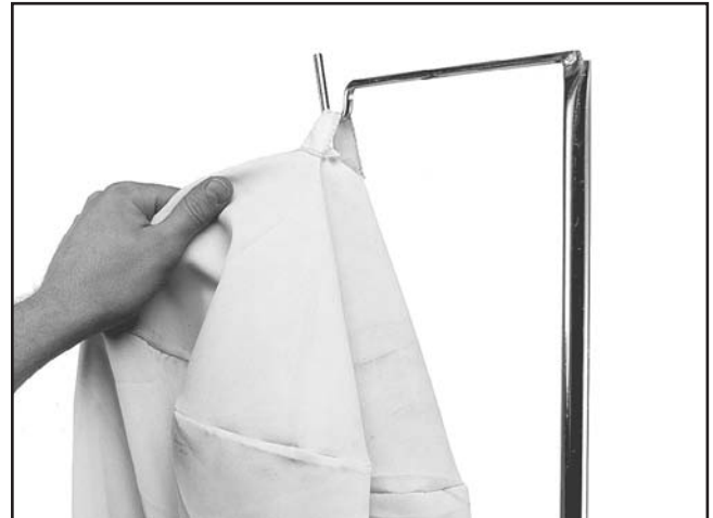
Figure 32. Attaching upper filter bag.
