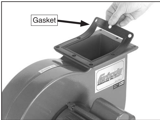
Figure 13. Positioning impeller outlet gasket.
