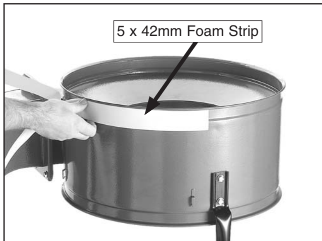
Figure 17. Applying the wide foam strip to the collector.
