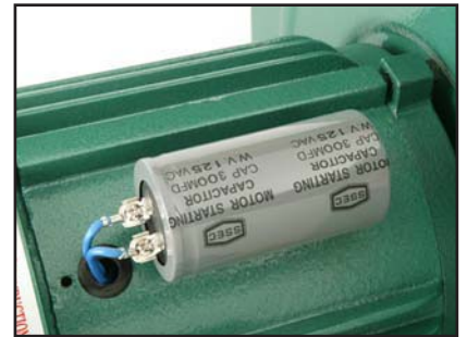
Figure 70. G0548Z start capacitor.
