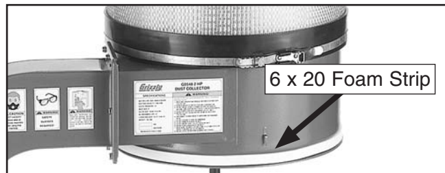
Figure 34. Example of 6 x 20 foam strip installed.
