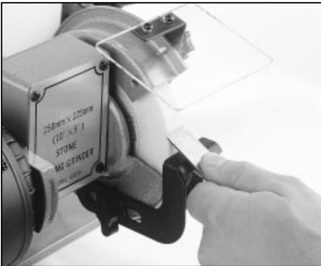
Figure 4. Proper grinding positioning.
