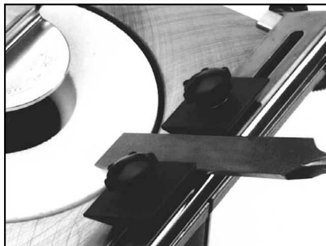
Figure 3. Stationary clamps in place.
