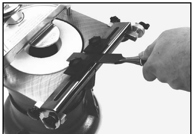
Figure 7. Stationary clamps holding chisel.
