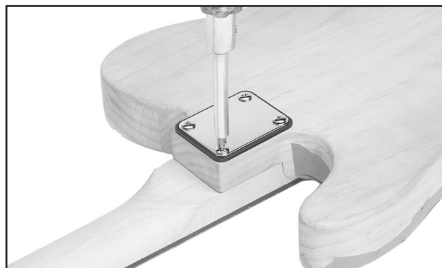
Figure 10. Fastening neck to body.
