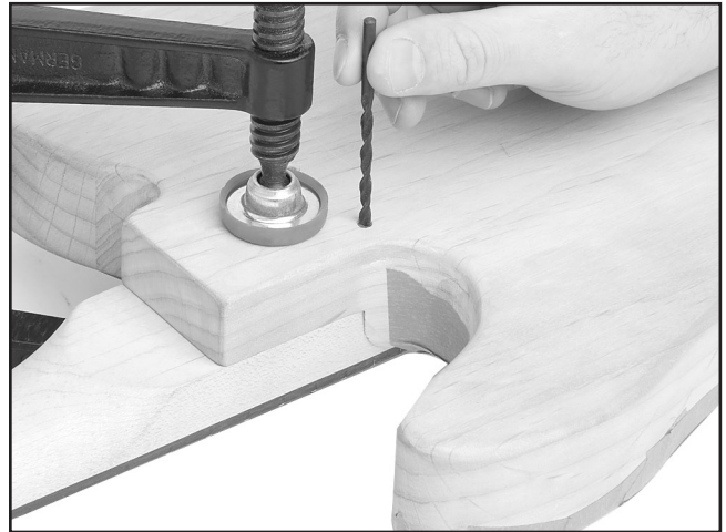
Figure 8. Making a pilot hole in the neck.
