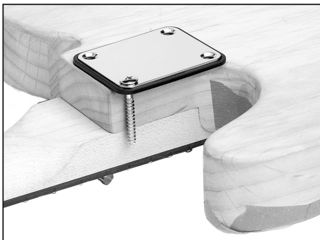
Figure 9. Using screw tip depth to set depth stop.
