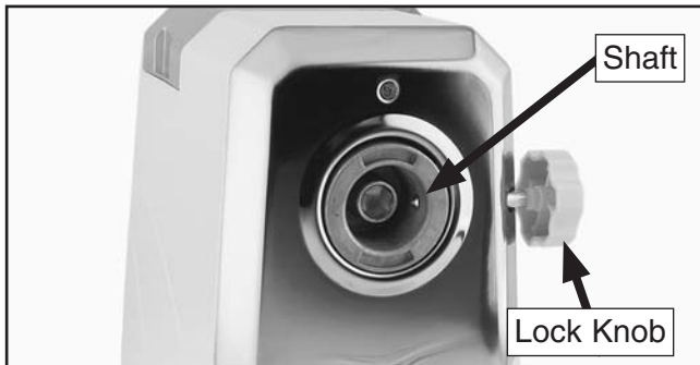
Figure 4. Lock knob shaft flush with inside of grinder.
