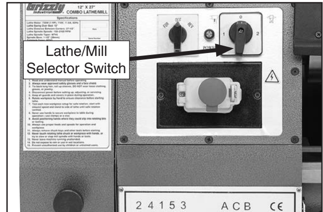
Figure 94. Location of lathe/mill selector switch.
