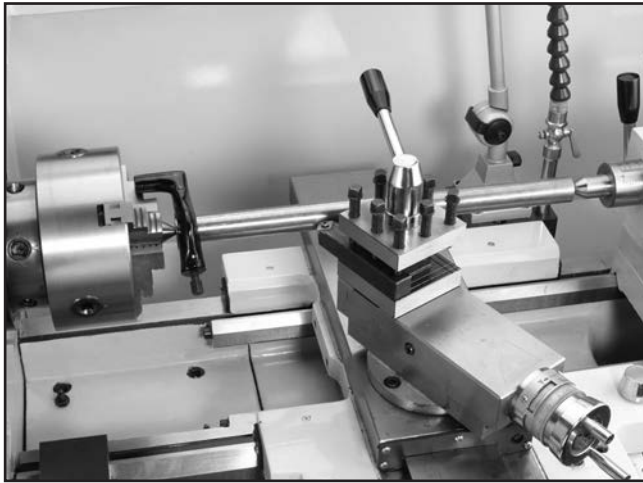
Figure 37. Example of stock mounted between the centers.
