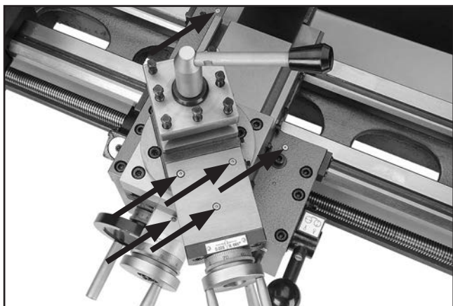
Figure 111. Apron ball oilers.
