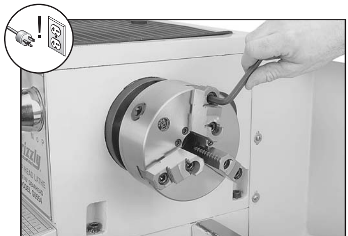
Figure 29. Loosening the jaw cap screws.
