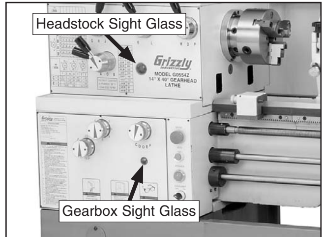
Figure 78. Headstock and gearbox oil sight glasses.
