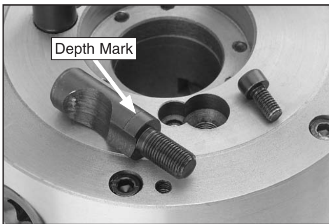
Figure 28. Cam-lock stud depth mark.
