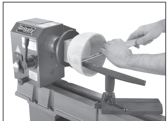
Figure 38. Typical faceplate turning operation.
