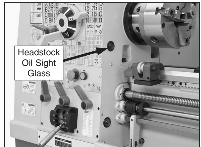
Figure 99. Location of headstock oil sight glass.
