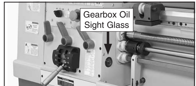
Figure 101. Location of gearbox oil sight glass.
