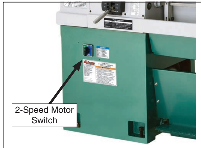
Figure 141. 2-Speed motor switch.
