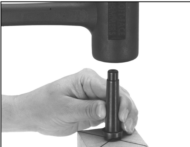
Figure 25. Seating the spur center.
