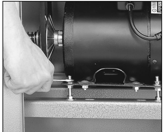
Figure 7. Loosening motor mount bolts.
