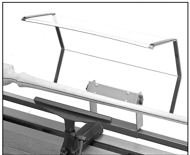
Figure 12. Guard assembly in place.
