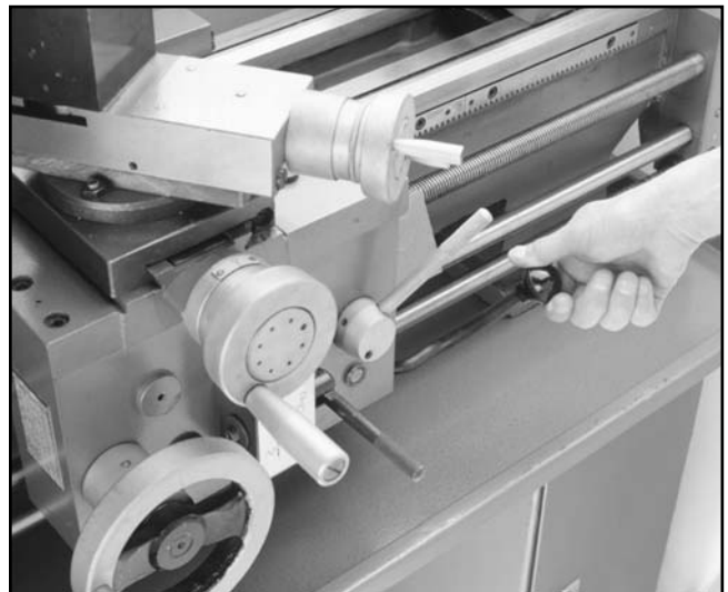
Figure 21. Spindle rotation control lever.
