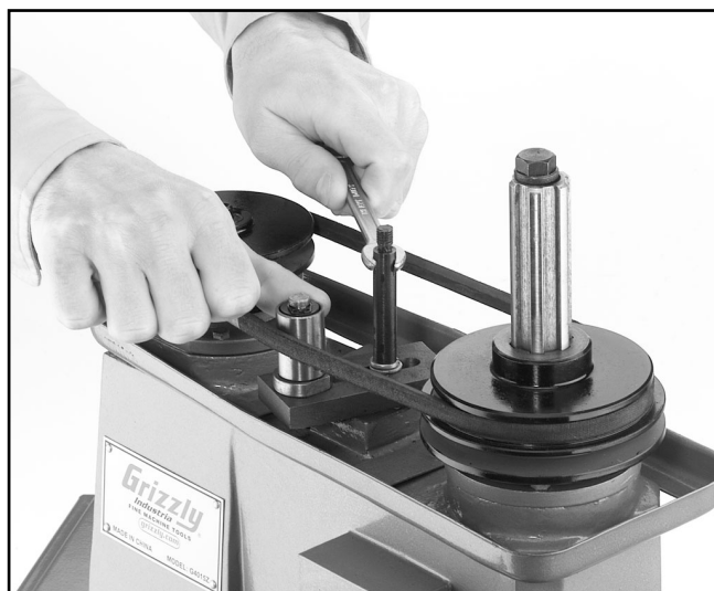
Figure 26. Loosen stud to pivot belt tensioner.
