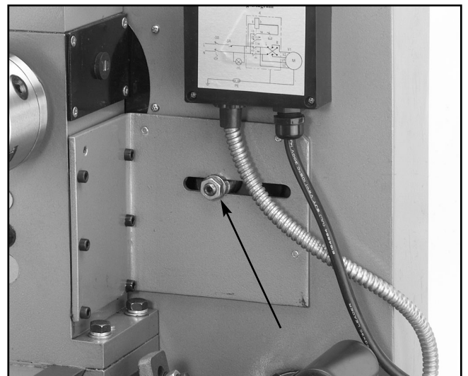
Figure 17. Loosen this nut to adjust pulley.
