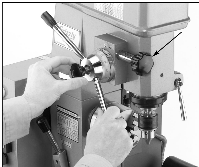
Figure 27. Move the handle while depressing knob.
