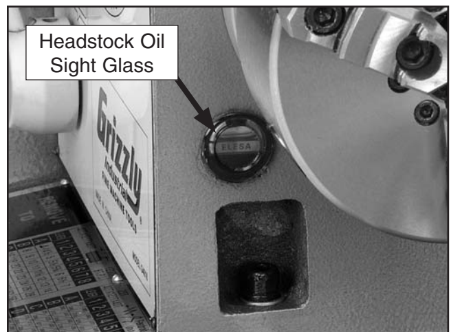
Figure 12. Headstock oil sight location.
