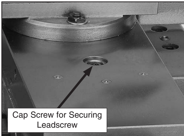
Figure 82. Cap screw securing the leadscrew.
