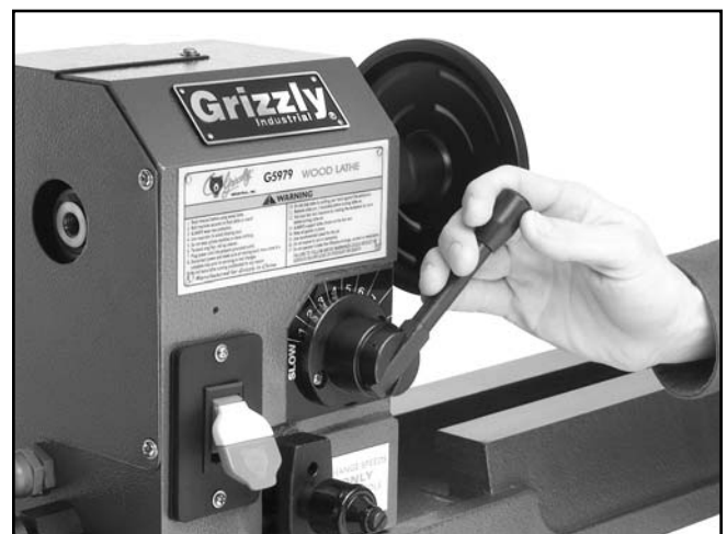
Figure 16. Adjusting spindle speed.
