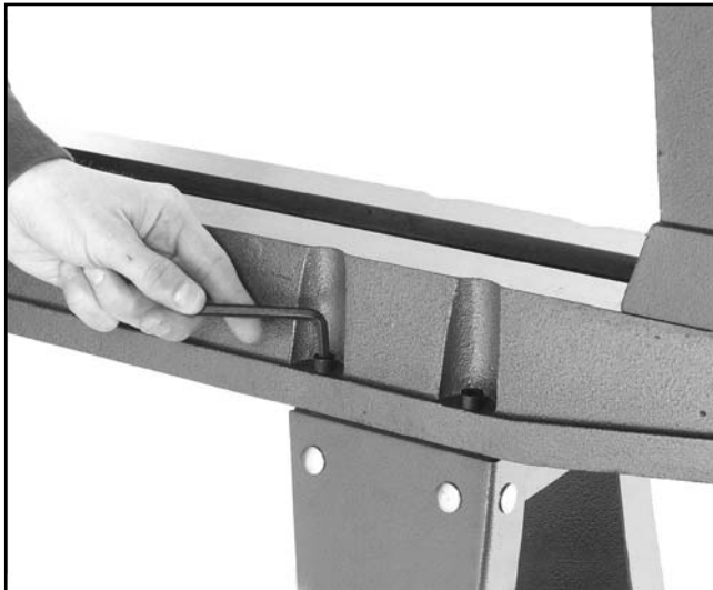
Figure 5. Attaching lathe unit to stand.
