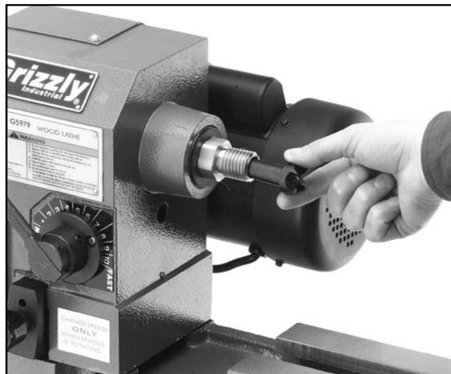
Figure 8. Installing the spur center.
