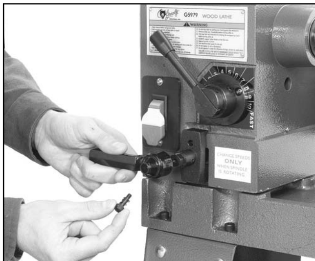
Figure 7. Attaching the headstock lock handle.
