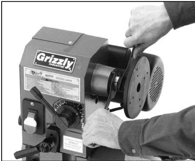
Figure 10. Attaching the faceplate.
