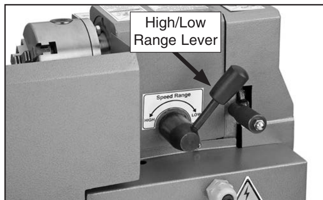
Figure 47. High/low range lever set to low.
