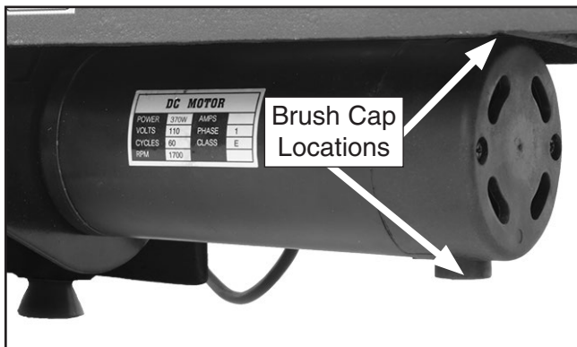
Figure 55. Motor brush cap locations.
