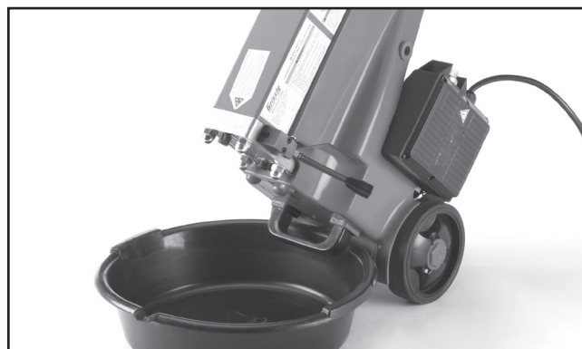
Figure 11. Draining hydraulic fluid.
