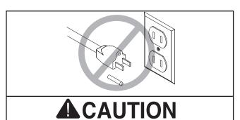
SHOCK HAZARD! The amplifier must have a ground prong in the plug to help ensure that it is grounded. DO NOT remove this prong to fit the plug into a two-pronged outlet!
