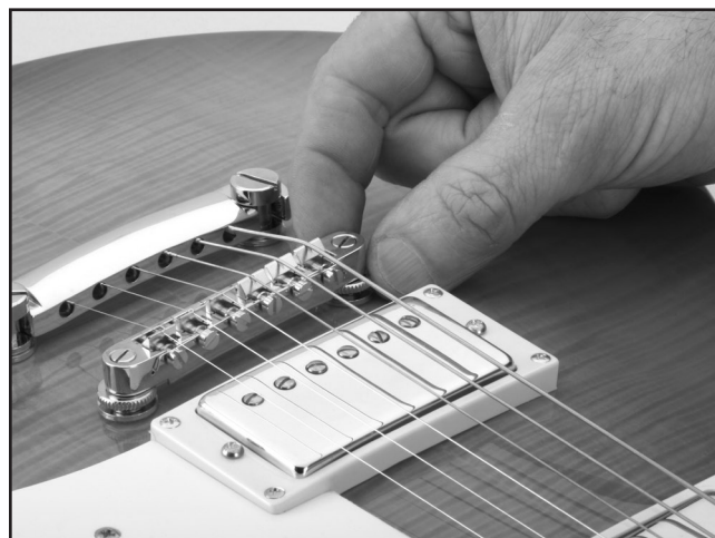
Figure 38. Adjusting the bridge height.
