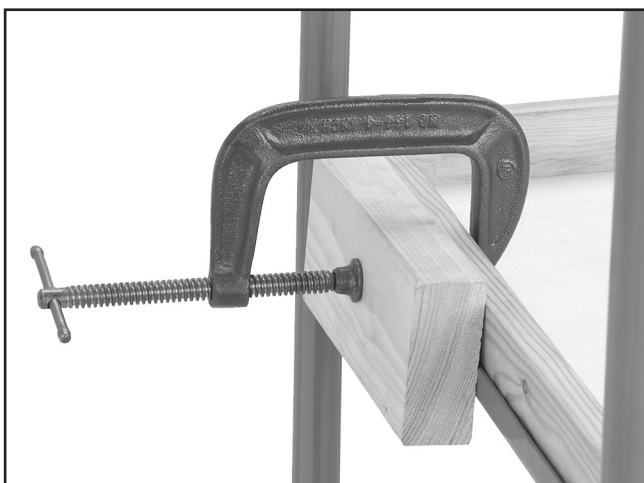
Figure 8. Using clamp to align mounting holes.
