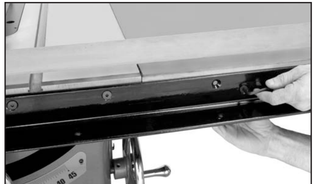
Figure 32. Aligning main extension table.
