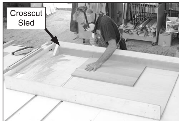
Figure 110. Example of crosscut sled.
