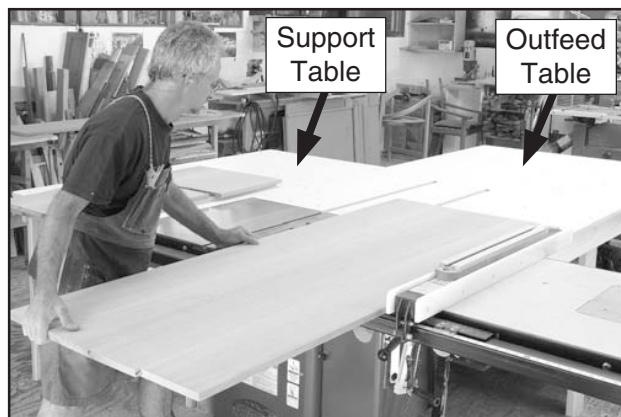
Figure 109. Example of outfeed & support tables.
