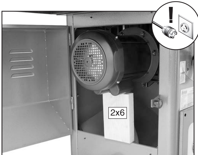
Figure 151. Motor resting on wood block.
