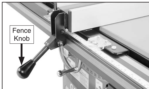
Figure 42. Fence knob installed.
