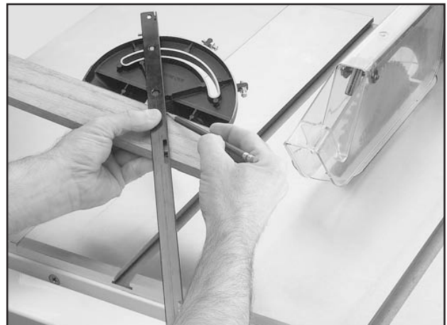
Figure 76. Example of marking miter line.
