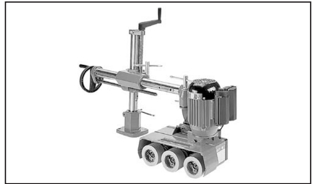
Figure 112. G4179 Power Feeder.
