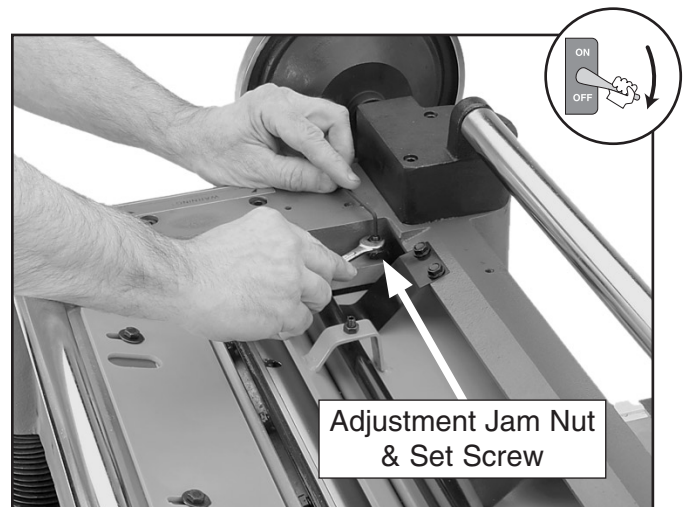
Figure 46. Adjusting the pressure bar height.
