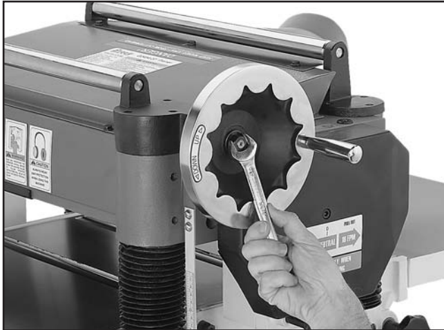
Figure 9. Installing the table height handwheel.
