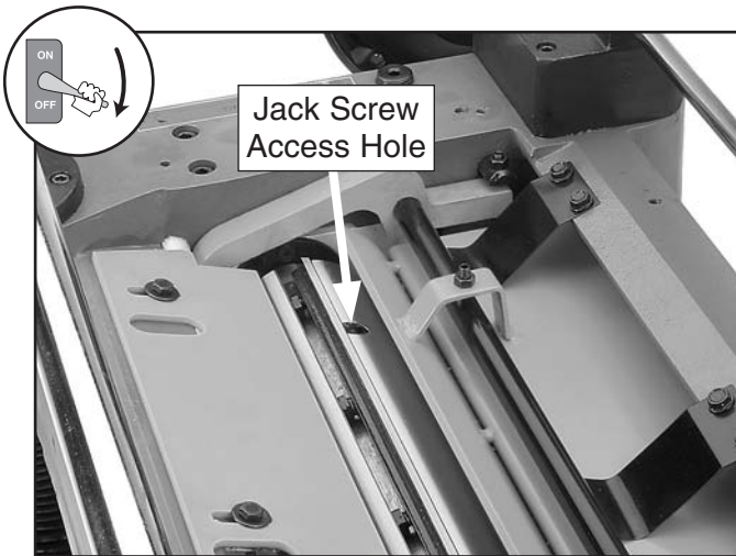
Figure 36. Jack screw access hole in the cutterhead.
