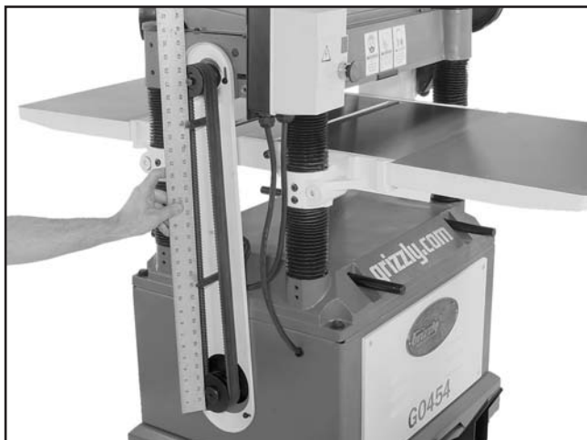
Figure 52. Checking pulley alignment.
