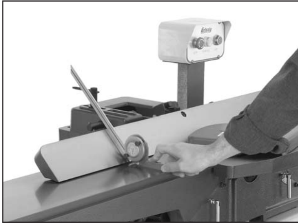
Figure 48. Typical 45° outward fence adjustment.
