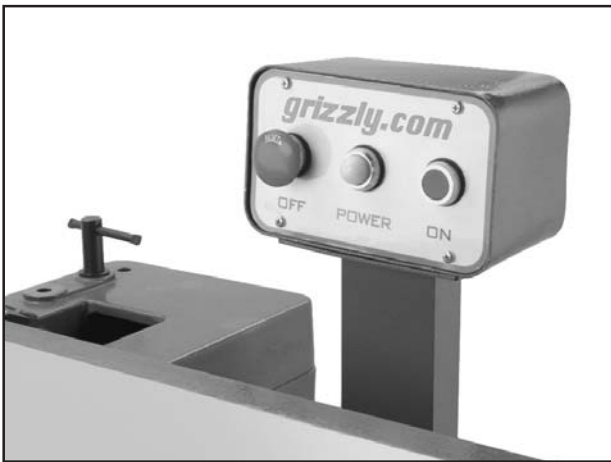
Figure 10. Switch positioned above the fence so it is accessible from the front.
