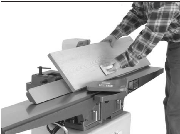
Figure 19. Typical bevel cutting operation.
