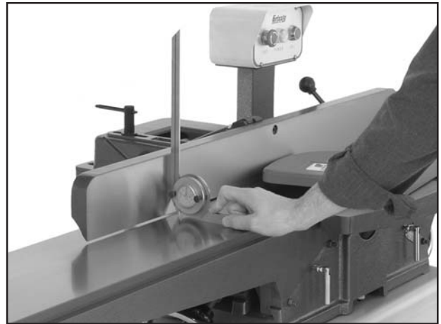
Figure 46. Typical 90° fence adjustment.
