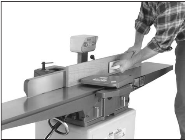
Figure 17. Typical edge jointing operation.
