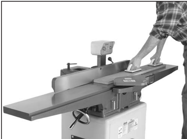
Figure 22. Typical surface planing operation.
