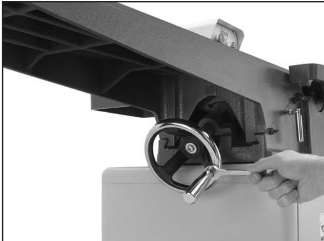
Figure 16. Securing the handwheel handle.
