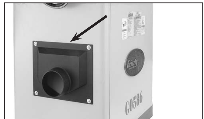
Figure 15. Correctly installed dust port.
