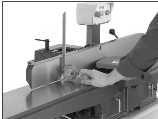
Figure 49. Adjusting fence to 90°.
