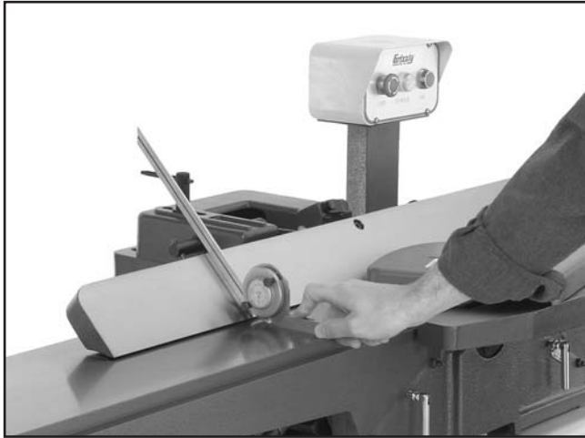
Figure 51. Adjusting fence 45° outward.
