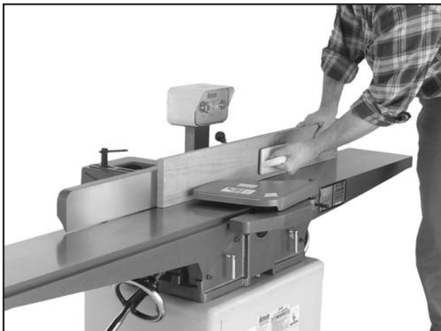
Figure 24. Typical edge jointing operation.
