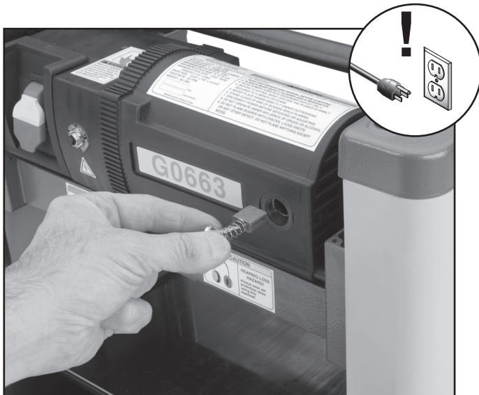
Figure 24. Brush holder location (another brush is located on the other side of the motor from the one shown in this picture).
