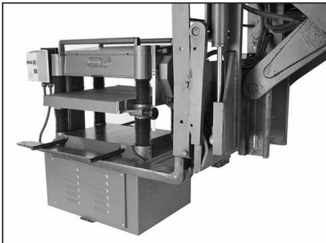
Figure 6. Example of planer being lifted using forklift.
