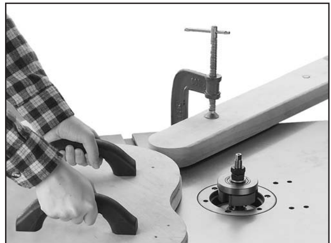
Figure 36. Example of using a jig with a starting block being used on a shaper.
