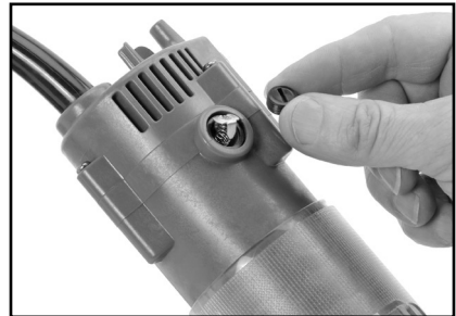
Figure 22. Replacing the motor brushes.
