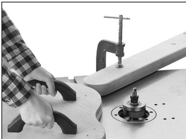
Figure 27. Example of using a jig with a starting block.
