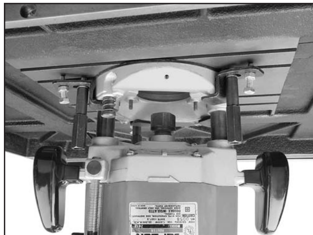
Figure 20. Router installed in the hold-downs.
