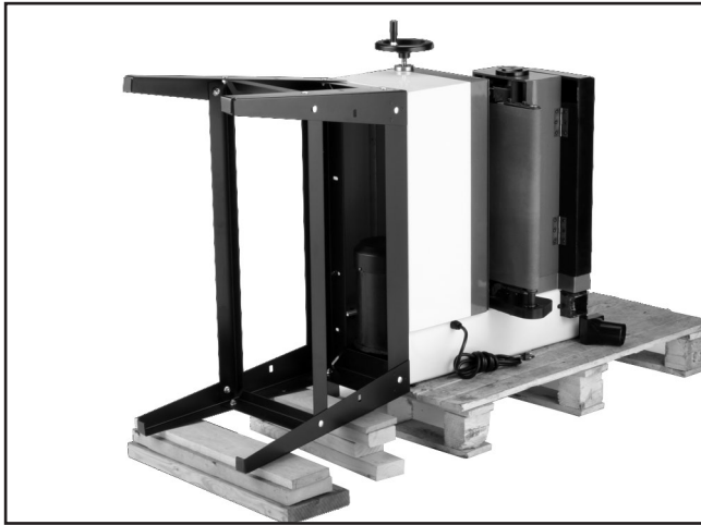
Figure 10. Stand resting on blocks.
