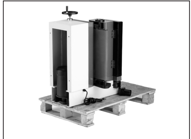
Figure 8. Sander tipped back on pallet against pulley cover.
