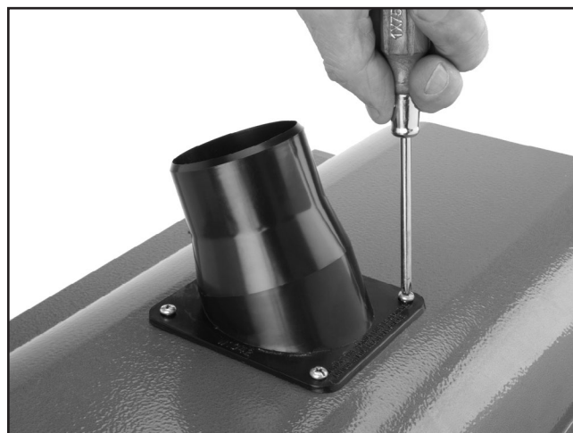
Figure 7. Dust port installation.
