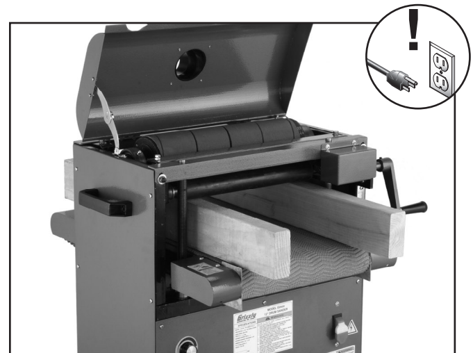
Figure 30. Gauge blocks positioned under pressure rollers and sanding drum.
