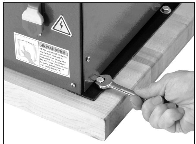
Figure 5. Installing sander onto bench top.
