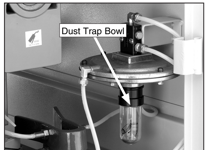
Figure 23. Unscrew the clear canister to empty the air line dust trap.
