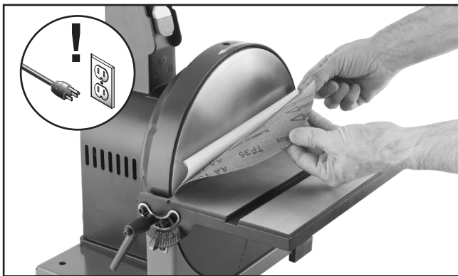
Figure 12. Sanding disc being slipped between the disc and table.
