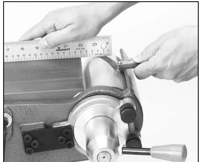
Figure 15. Measuring platen to roller parallelism.
