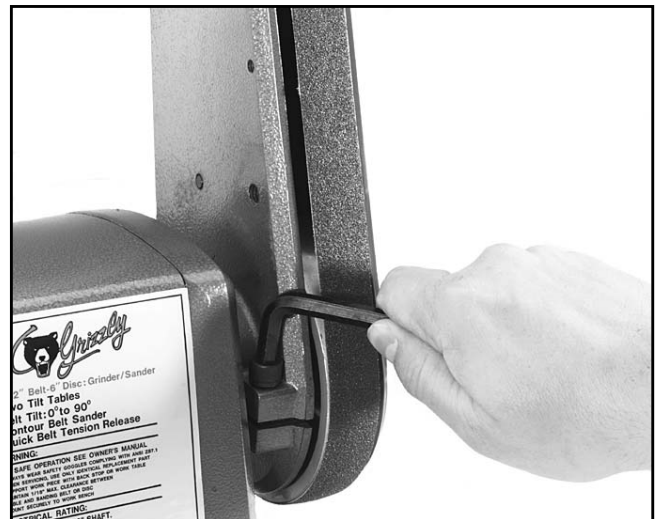
Figure 9. Horizontal tilt of belt sander.
