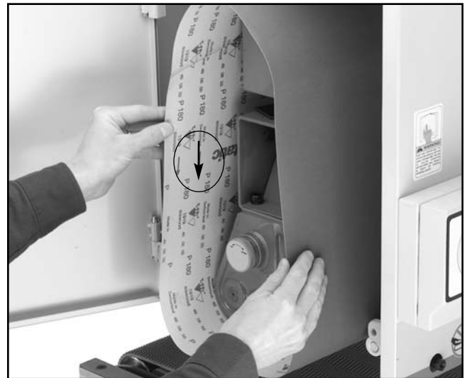
Figure 11. Place belt over the three belt rollers to install. Make sure arrows on inside of belt point in the direction of rotation.
