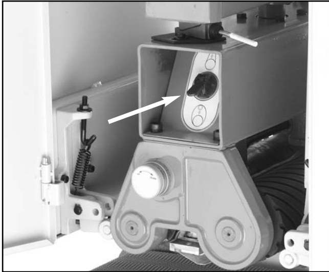
Figure 12. This is the belt tension switch.
