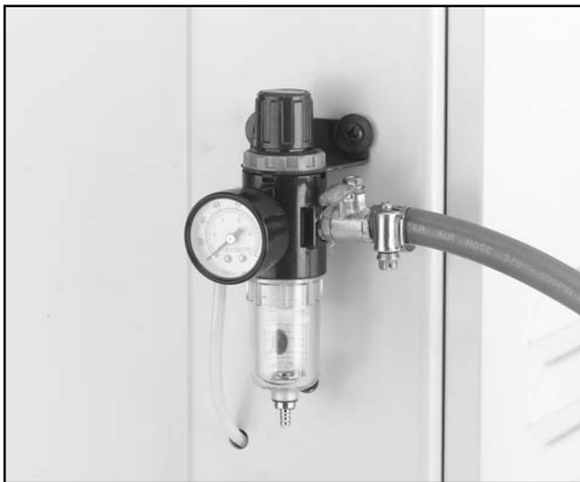
Figure 10. Secure air hose with a hose clamp.
