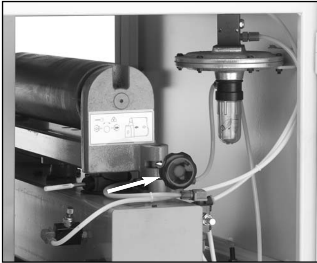
Figure 20. This is the oscillation timing control knob.
