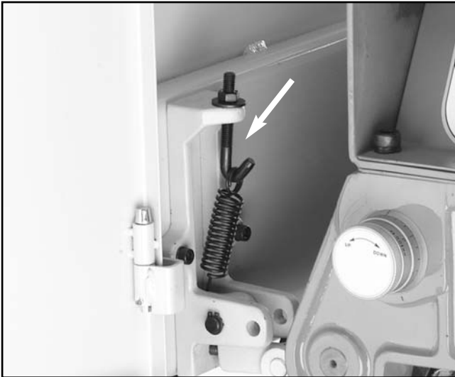
Figure 25. This is one of the four pressure roller adjustment bolts.
