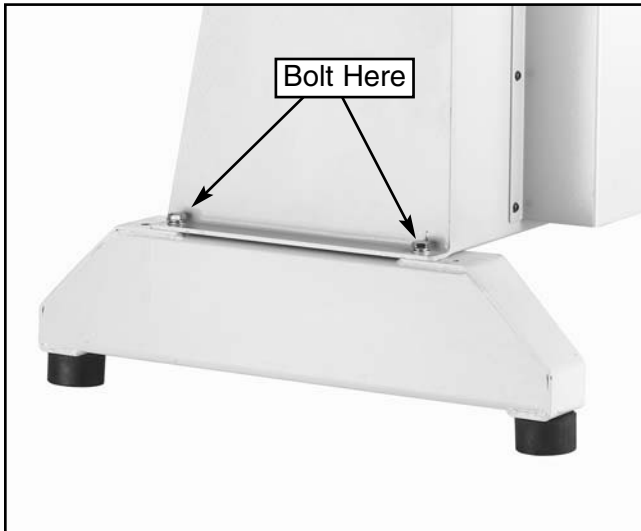
Figure 7. Attaching base supports to main base.
