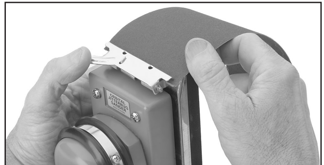
Figure 2. Attaching sanding sheet.
