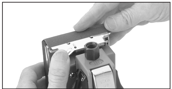
Figure 3. Attaching sandpaper on opposite side.
