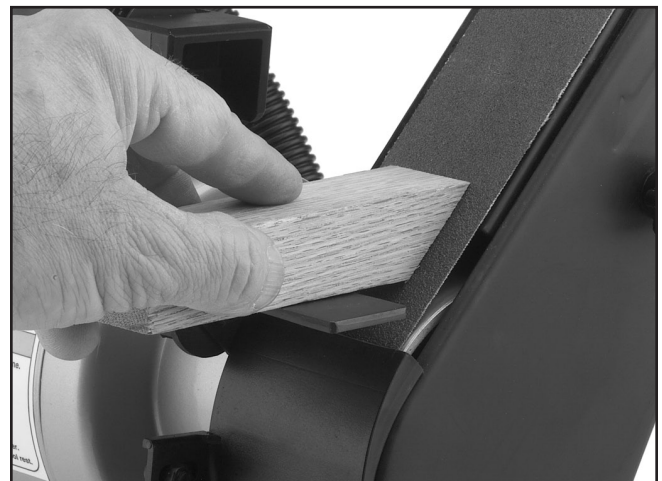
Figure 15. Sanding a workpiece.
