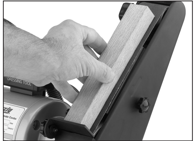
Figure 14. Sanding a workpiece.
