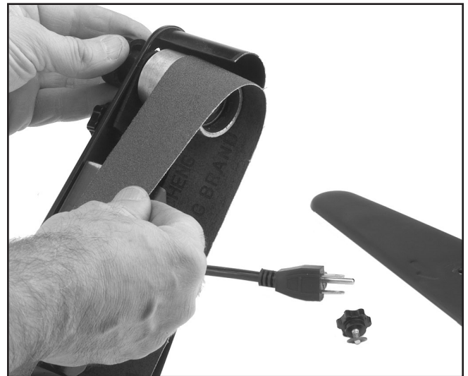
Figure 18. Removing sanding belt.
