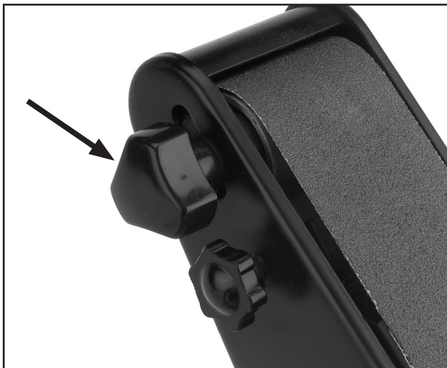
Figure 17. Sanding belt tension knob.
