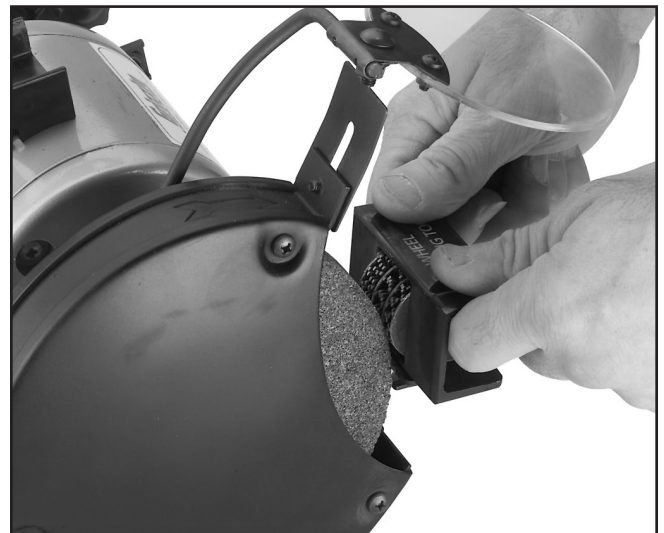
Figure 10. Using wheel dressing tool.
