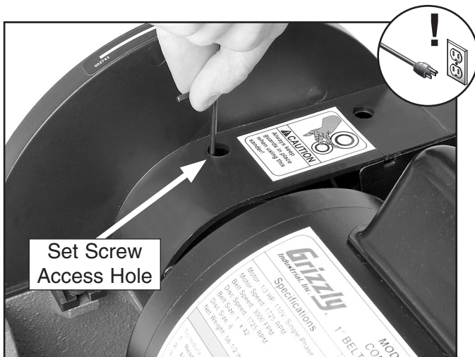
Figure 13. Securing the sanding disc set screw.
